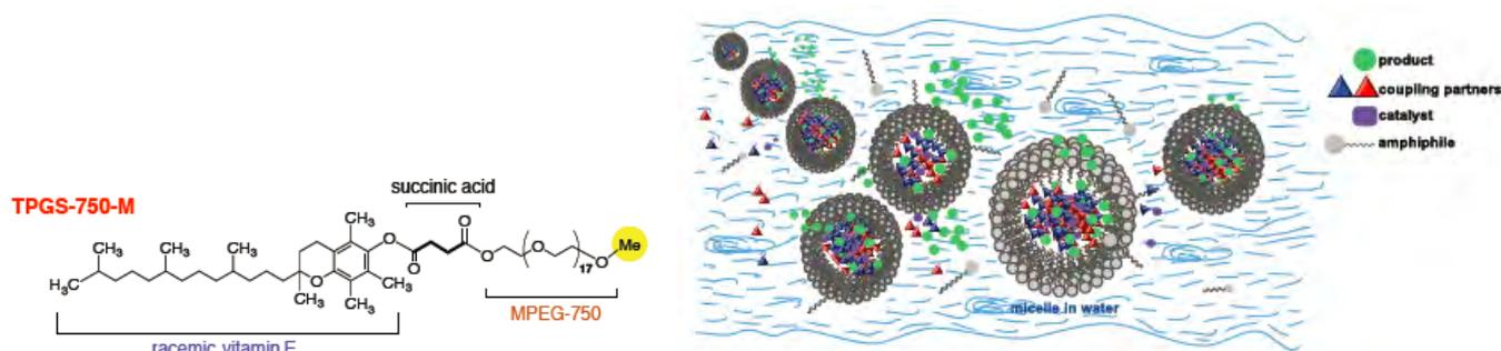
Modern no-ionic surfactants for micellar catalysis in water.
