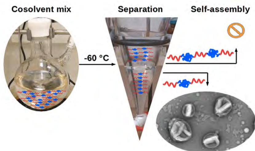
**Figure 1.** Schematic illustration of the cosolvent extraction enabling the separation polymersome forming triblock copolymers from multiblock copolymers.
